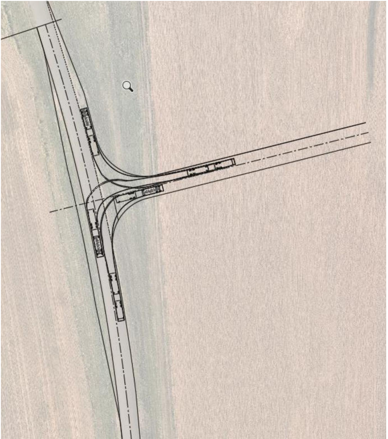
Figure 3.10 – Proposed Gowrie Road & Quarry Access Intersection – Swept Path Analysis, BAL/BAR Treatment (Tipper and TriAxle Dog Design Vehicle) [Page 25, Traffic Impact Assessment].
